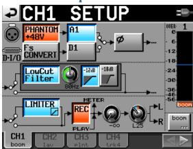
As described in Part 1, go to the **Channel Setup** screen in the **MENU** section. Select the appropriate parameters for each input channel that you are using, such as Phantom on/off, and so on. At this stage, you do NOT need to worry about arming the track, nor adjusting the pan and output levels. Those tasks can be done from the HOME screen later on.
