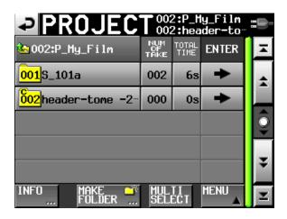
go to the PROJECT screen either by pressing the scene/take box just above the meters on the HOME screen, or by pressing the PROJECT button. Then, just press the name of your project, and the screen will advance to display all of the scenes within it. You will see the MAKE FOLDER tab at the bottom of the screen.
