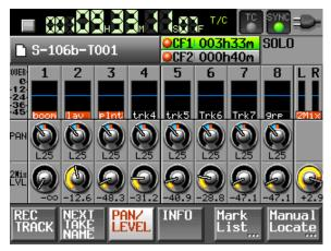
The **PAN LEVEL** tab is where you would normally access the **OUTPUT LEVEL** and **PAN** controls for each input channel. Pressing the virtual knob will link it to the physical **DATA** knob on the recorder. An advantage of using this screen instead of the Channel Setup screen for these functions is that the PAN LEVEL screen shows meters for each channel as well as the master LR mix.
