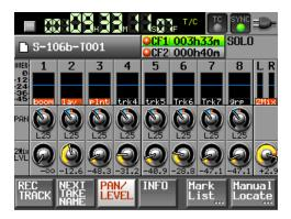
Select the **PAN LEVEL** tab at the bottom of the **HOME** root screen. Using the virtual knobs, assign each input to L100 (aka 100% left) or R100 (aka 100% right), if you are recording a discreet two-track dialogue mix for film/video.
