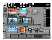
On the lower right of the Channel Setup window is a button with the track name or label, just under the level meter. Pressing that button allows you to instantly rename the track display to something more meaningful, such as changing "Track 2" to "Boom", or "Track 5" to "Brad".
