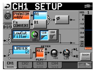
The screen of the **Channel setup** window shows tabs for input channels 1-4. Selecting the arrow tab on the right will bring up channels 5-8, and vice versa.
